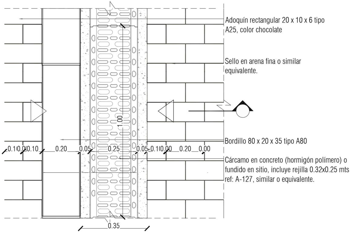
CORTE: CÁRCAMO EN CONCRETO A-127 ESC: 1:10
