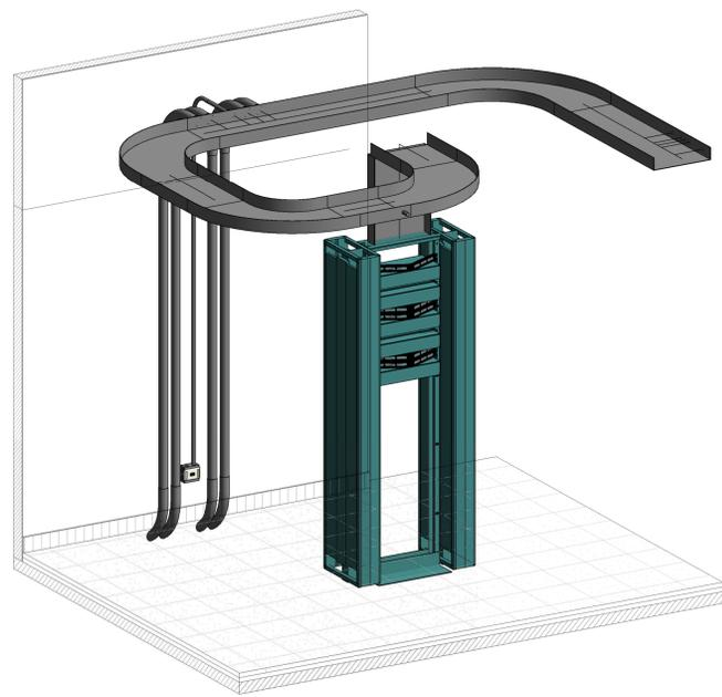
3 DETALLE 3D SISTEMA CABLEADO ESTRUCTURADO
