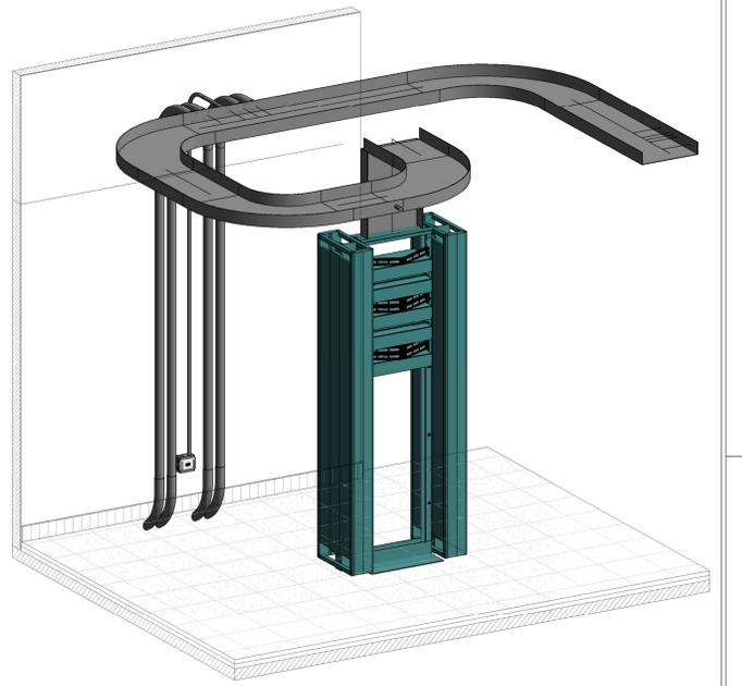
3 DETALLE 3D SISTEMA CABLEADO ESTRUCTURADO
